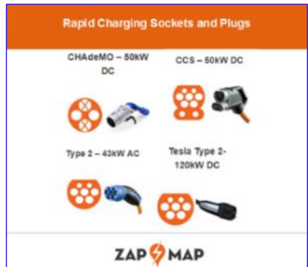
Figure 5: Charging sockets and plug types (Source: Zap-Map)
