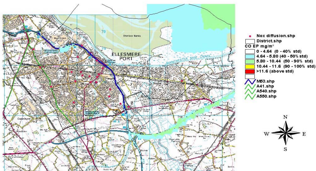
Figure 10 Small-scale map areas of 2003 predicted 8-hour mean CO concentrations in EPNBC area (NAQS objective - running 8 hour mean - 11.6 mg/m 3 )
