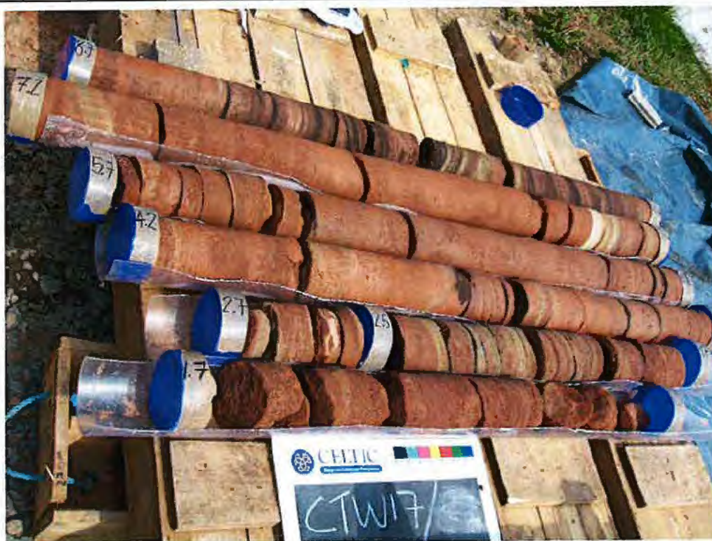
Plate No.: 50 Title: Core Samples Recovered from Treatment Well CTW17
