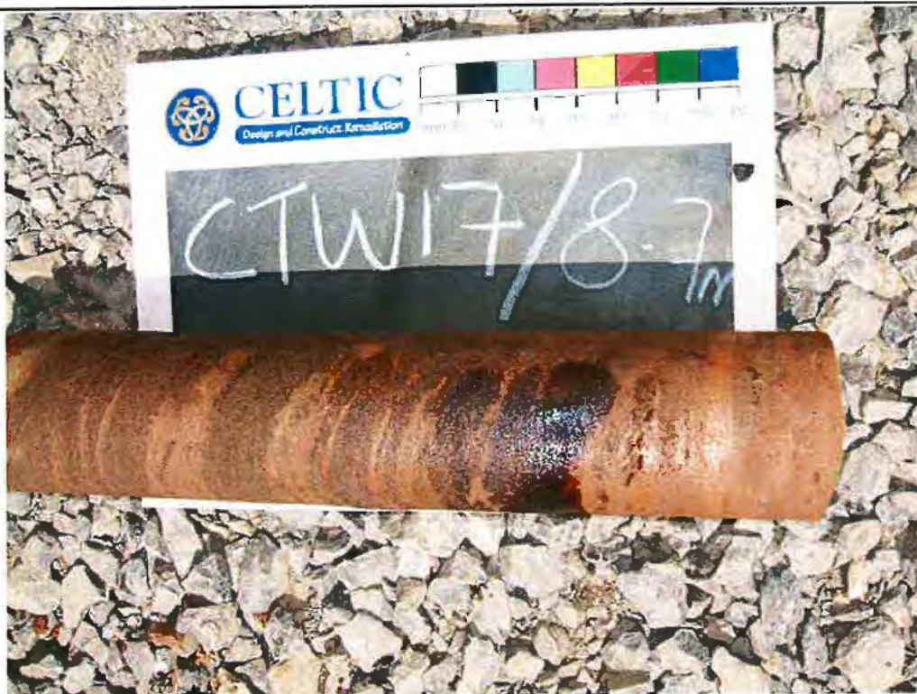
Plate No.: 49 Title: Core Sample Recovered from Treatment Well CTW17 Shows Heavy NAPL Staining
