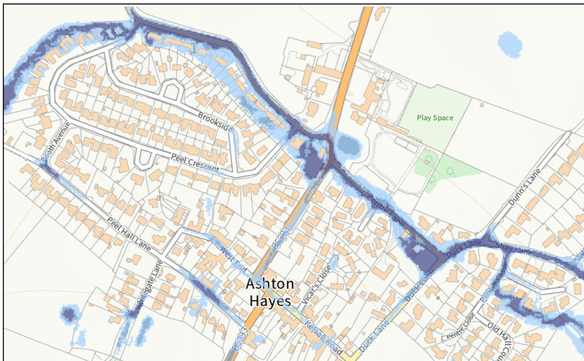
Extent of flooding from surface water
