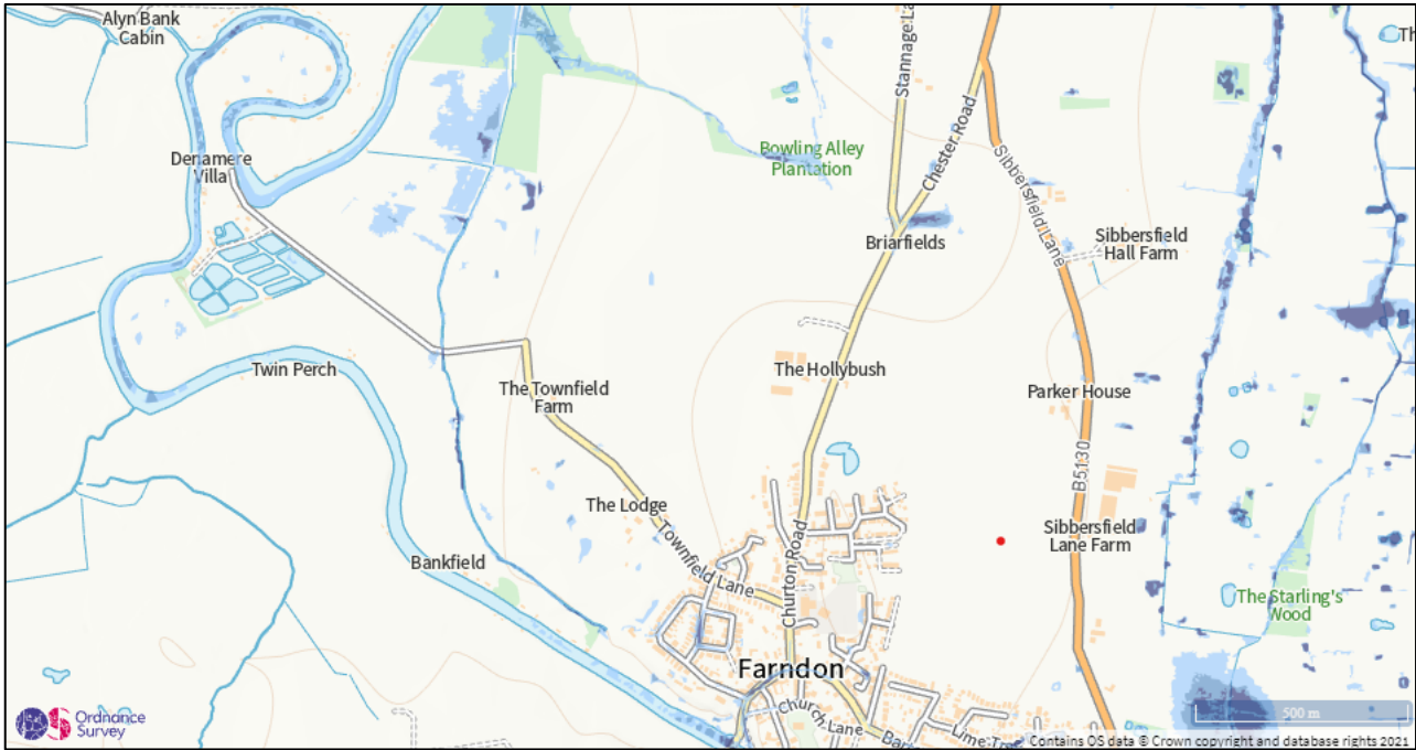
Extent of flooding from surface water
