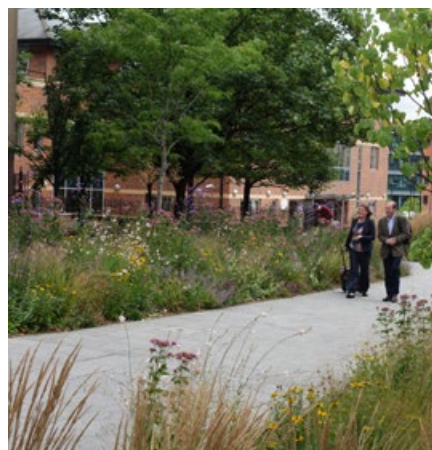
Example of attractive planting for a Sustainable urban Drainage System in Sheffield
