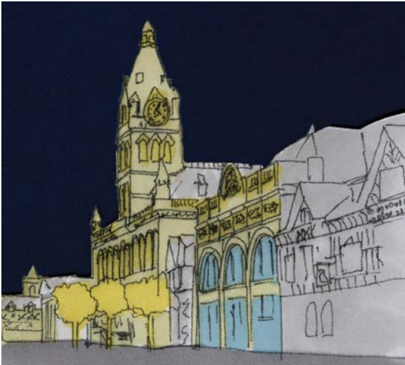
Proposed lighting scheme to entire Town Hall using combination of close offset lighting and gentle floodlighting
