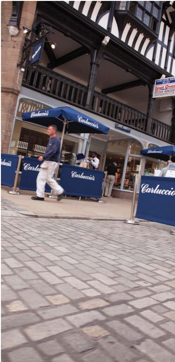
Example of appropriate aesthetic and quality for temporary barriers (Posts and bases must be robust enough to withstand strong winds and tapping rail must be included)
